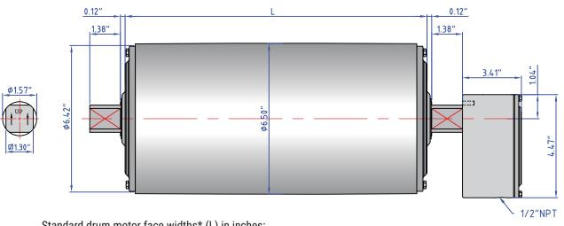
NOTE: Junction Box does not rotate. Power entry at 6 o'clock position.
