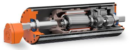
The input power cable passes through the hollow shaft and is connected to the motor stator. The electric motor is mechanically connected in-line to the gear reducer. The drum motor is partially filled with oil. The oil inside the drum motor lubricates all mechanical components and helps to dissipate heat generated by the electric motor and gear reducer onto the drum, and from the drum to the belt. In theory, the drum motor is cooled by the belt making full contact with the rotating steel drum.
