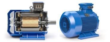
In order for an electric motor to produce rotation, a rotating electromagnetic field is needed. To achieve that, it requires ferrous and nonferrous materials, such as iron and copper or iron and aluminum. The stationary part of an electric motor (the stator) has motor windings that are copper and a laminated stator core that is iron. The rotating part (the rotor) of the electric motor is made up of iron laminations and aluminum bars.
